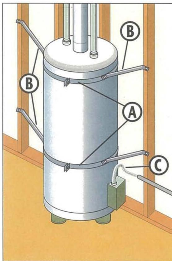
Wrap a 1-1/2-inch-wide, 16-gauge-thick metal strap (A) around the top of the water heater and bolt the ends together. Do the same about 1/3 of the way up the side of the water heater. Take four lengths of EMT electrical conduit, each no longer than 30 inches. Flatten the ends. Bolt one end to the metal strap as shown (B). Screw the other end to a 2-inch by 4-inch stud in the wall using a 5/16-inch by 3-inch lag screw. Be sure a flexible pipe (C) is used to connect the gas supply to the heater.
