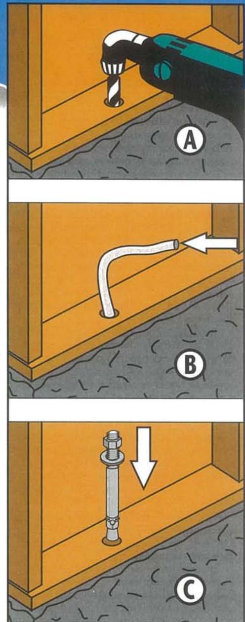
Bolting the wood frame of an older house to the concrete foundation can significantly reduce earthquake damage. Every 3 to 4 feet along the foundation, drill a hole using a right-angle drill with a 1/2-inch bit (A), blow the concrete powder out of the hole with a small piece of flexible tubing (B), and hammer in an expansion bolt, 1/2-inch in diameter and about 7-1/2 inches in length (C). Tighten the nut on the expansion bolt.
