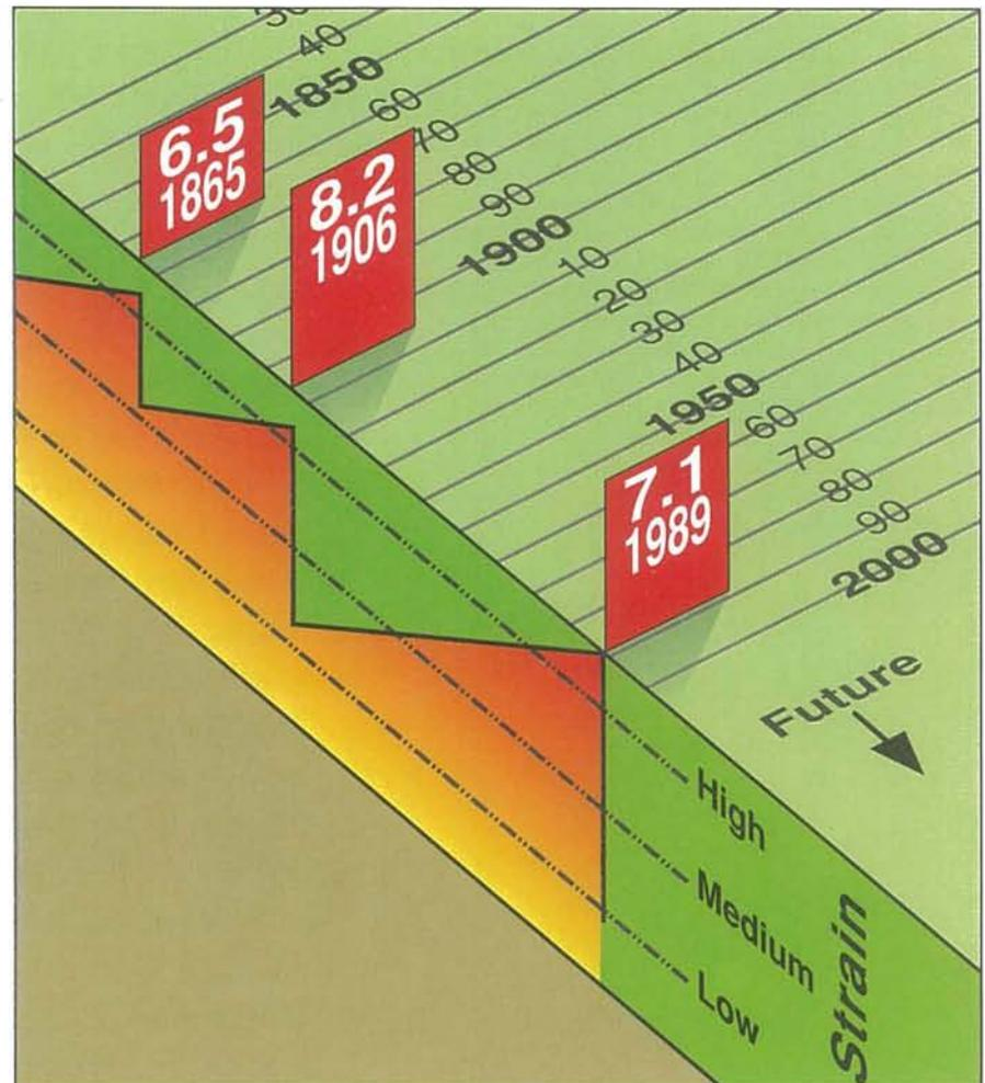
Along the San Andreas fault in the Santa Cruz Mountains, strain appears to increase at an average rate of 0.75 inches per year. This strain was reduced by sudden fault slips during the magnitude 6.5 and 8.2 earthquakes in 1865 and 1906. In 1981, scientists estimated that the strain was at a high enough level to cause an earthquake and that this earthquake was likely to occur before 1996. The magnitude 7.1 Loma Prieta earthquake in 1989 proved their projections correct.
