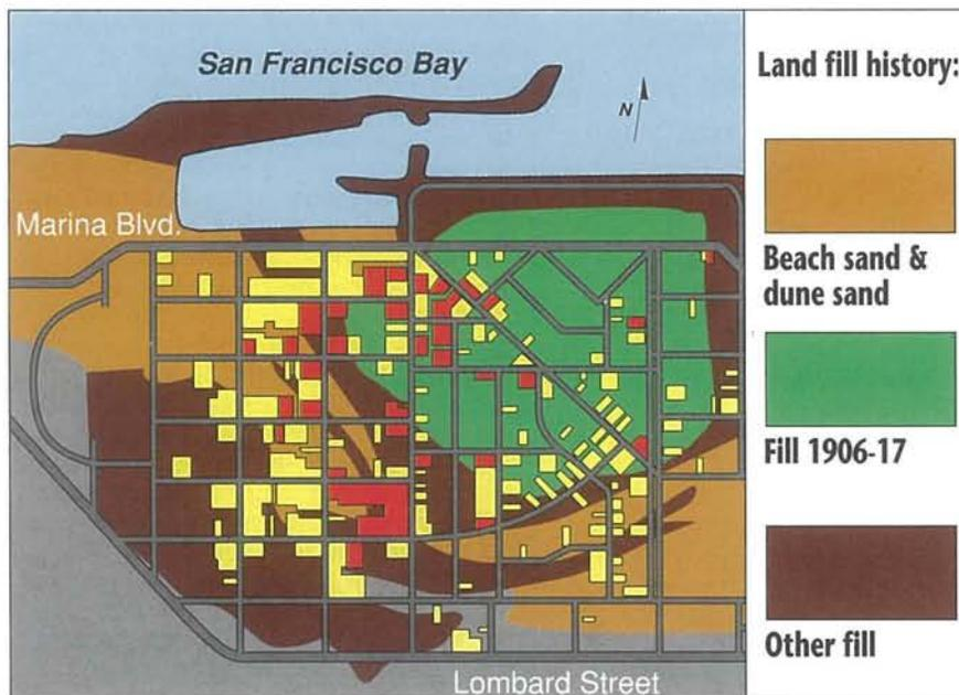
In the Marina District of San Francisco, maximum ground subsidence of as much as 5 inches was centered in the land filled between 1906 and 1917. Damage to buildings was greatest where filled land overlaps old beach sands. Demolished or severely damaged buildings are shown in red. Less damaged but uninhabitable buildings are shown in yellow.
