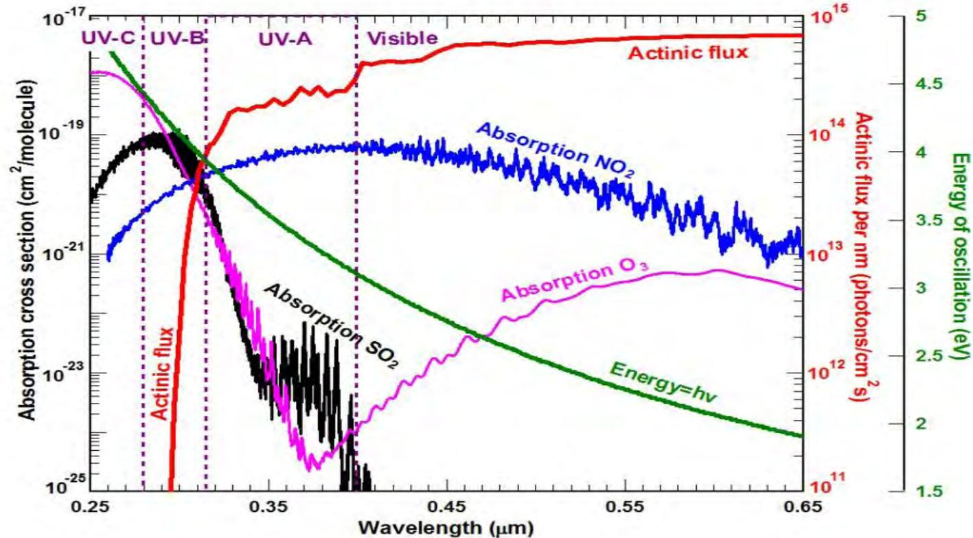
Note the very high absorption in the UV-A and UV-B bands where energy is rising rapidly and the actinic flux at the earth's surface is decreasing rapidly
