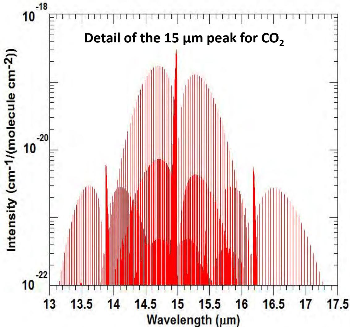
Each spectral line has a finite width and is typically assumed to have a Lorentz line shape
