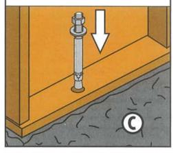
Bolting the wood frame of an older house to the concrete foundation can significantly reduce earthquake damage. Every 3 to 4 feet along the foundation, drill a hole using a right-angle drill with a 1/2-inch bit (A), blow the concrete powder out of the hole with a small piece of flexible tubing (B), and hammer in an expansion bolt, 1/2-inch in diameter and about 7-1/2 inches in length (C). Tighten the nut on the expansion bolt.
