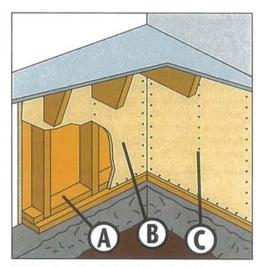
Reinforcing the "cripple" walls between the foundation and first floor of an older, wood-frame house can significantly reduce earthquake damage. Nail 2 by 4 inch blocks of wood to the mud sill as needed (A). Cut 1/2-inch plywood to fit the inner side of the wall (B). Fasten plywood along all edges and to each stud using 8d nails spaced 3 inches apart.
