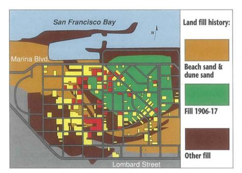
In the Marina District of San Francisco, maximum ground subsidence of as much as 5 inches was centered in the land filled between 1906 and 1917. Damage to buildings was greatest where filled land overlaps old beach sands. Demolished or severely damaged buildings are shown in red. Less damaged but uninhabitable buildings are shown in yellow.
