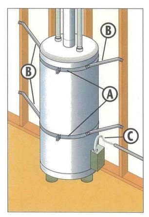
Wrap a 1-1/2-inch-wide, 16-gauge-thick metal strap (A) around the top of the water heater and bolt the ends together. Do the same about 1/3 of the way up the side of the water heater. Take four lengths of EMT electrical conduit, each no longer than 30 inches. Flatten the ends. Bolt one end to the metal strap as shown (B). Screw the other end to a 2-inch by 4-inch stud in the wall using a 5/16-inch by 3inch lag screw. Be sure a flexible pipe (C) is used to connect the gas supply to the heater.
